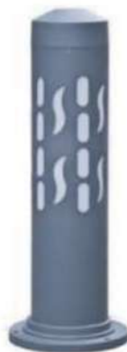
PRODUCT CODE 1688 DAZO POWER 10W, 15W, CCT 3000K, 4000K, 6000K MATERIAL TYPE M.S/ S.S / ALUMINIUM POWDER COATED HEIGHT 600 MM, 900MM, 1200 MM MRP
